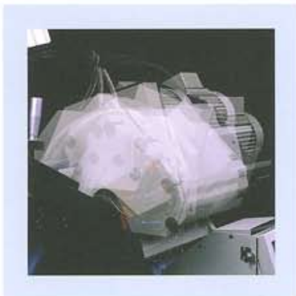
Grinding Wheel Head is turning over in process
