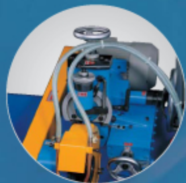
JF-330 Micro-adjustment for wheel head angle
