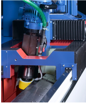
Type 5 VKA Back Micro Bevel as done on Softwood Veneer Peeling & Hardwood Veneer Slicing
